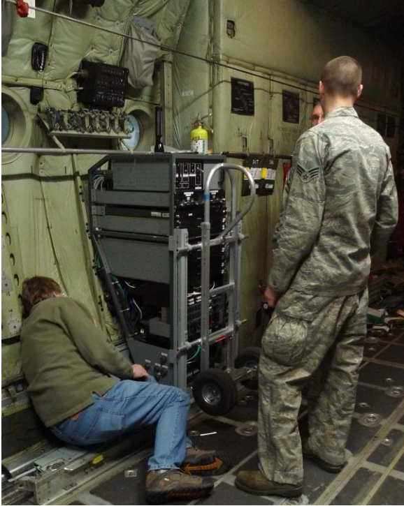
Avionics Rack being installed forward of the port side rear troop door
